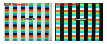
The same 2 patterns are also useful for Video-over-UTP Category cable both for the high-frequency loss compensation (above paragraph), but also for Skew Compensation for those devices that give you this flexibility. The right and left edges of the RGB bars should vertically line-up. Again, this pattern gives you a convenient means for making this adjustment.
